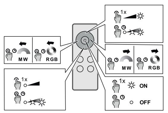
[Image 6] Connect Mesh Remote Eco, Operating concept
