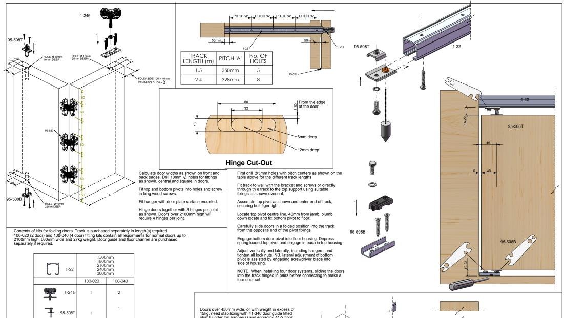
Doors over 450mm wide, or with weight in excess of 15kg, need stabilizing with 41-346 door guide fitted plumb under top hanger(s) and engaging 41-2 floor channel. Minimum door thickness must be 30mm. (Not included in standard kits).
