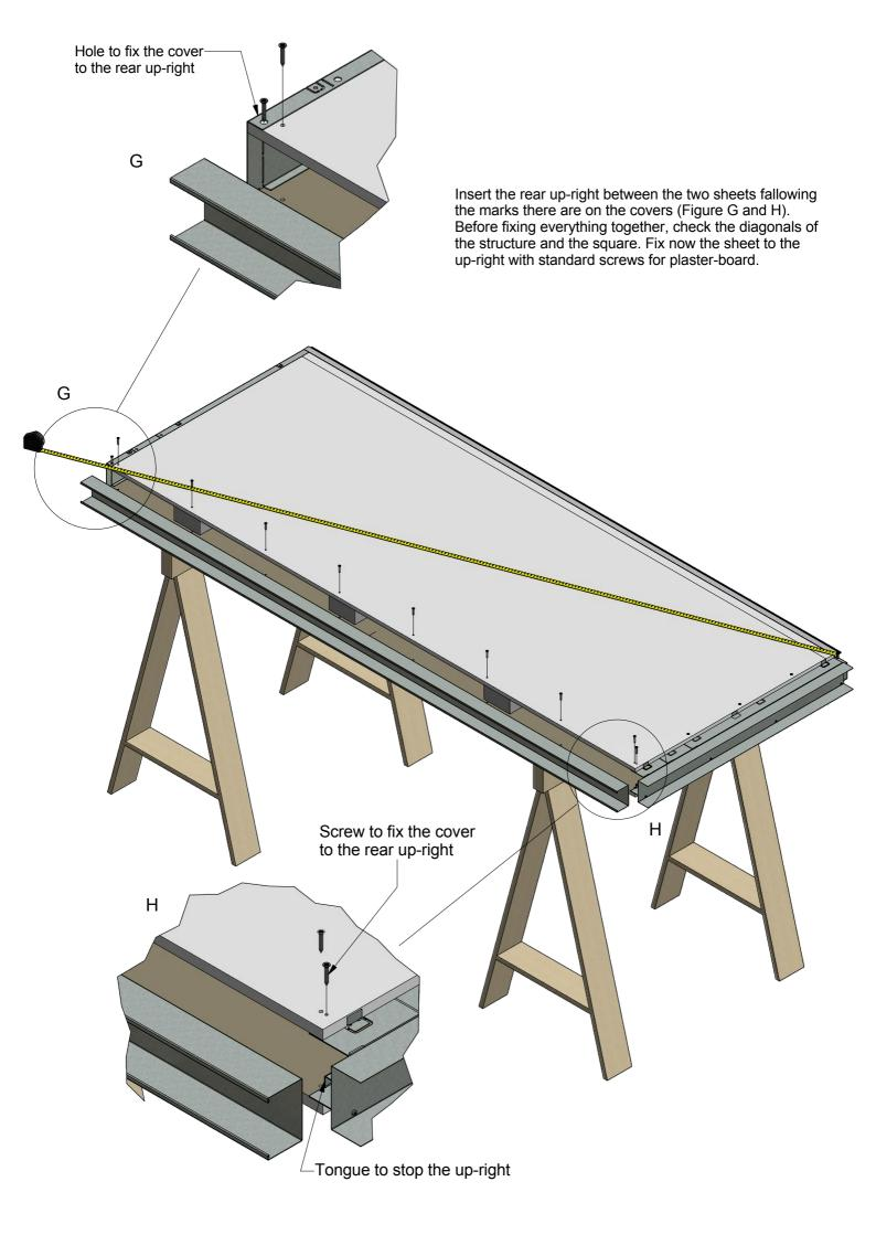
Fix now the the frontal cover to the aluminium profiles, always checking the diagonals of the structure and the square. The cover has to be inserted keeping the sliding accessories box inside the structure and the lower part aligned to the cover.
