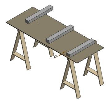
Place the second sheet on the polystyrene spacers aligned to the sheet below.
