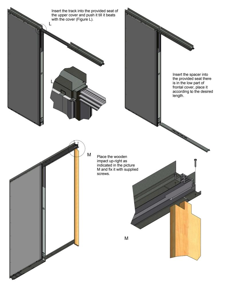
After the installation and when the wall is finished, is possible to install the door; to do it is necessary to remove the frontal cover and its screws, to remove also the lower spacer and the fixing screw of the wooden up-right.
